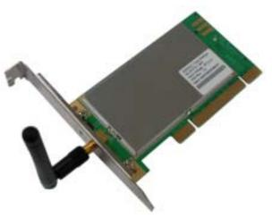
The WPG2000 can be used in ad-hoc mode to connect directly with other 2.4GHz wireless computers for peer-to-peer file sharing; or in infrastructure mode to connect with a wireless access point or router for accessing to the Internet in your office or home network.
